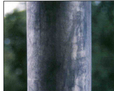
Mottled appearance when light grey pure zinc is surrounded by dark grey zinc-iron alloys developed, for example where reaction is greater at grain boundaries and locally allows the full thickness of coating to convert to zinc-iron alloy.
